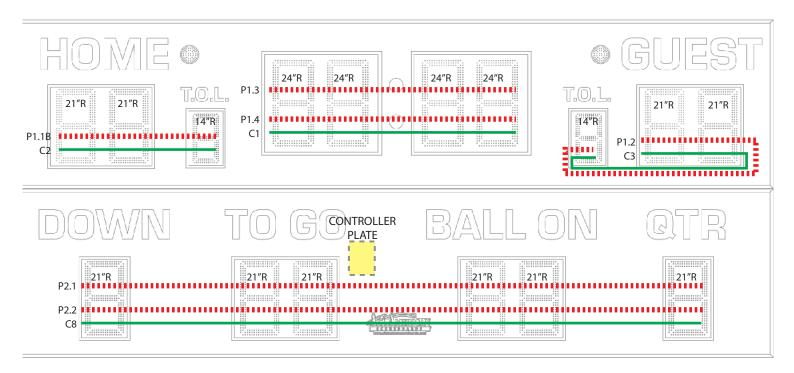
Power Supply Outputs (Full Brightness & Full Digits): P1.1≈4.23A P1.2≈2.81A P1.3≈2.81A P1.4≈3.57A P2.1≈3.90A P2.2≈3.90A
