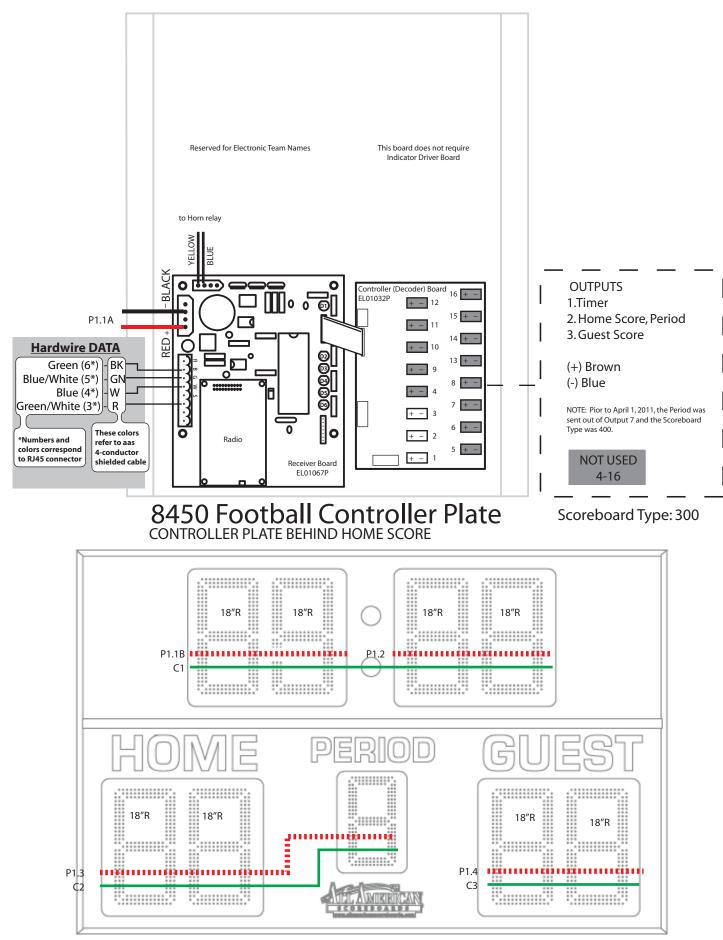
Power Supply Outputs (Full Brightness & Full Digits): P1.1≈2.98A P1.2≈2.38A P1.3≈3.48A P1.4≈2.38A "C" refers to controller board output. If Indicators are used, C4 data will go to the Indicator Driver Board and then to the digit(s). = DATA = DATA = 10.5VDC POWER = 115 VAC / 60 Hz - 3.0 Amps
