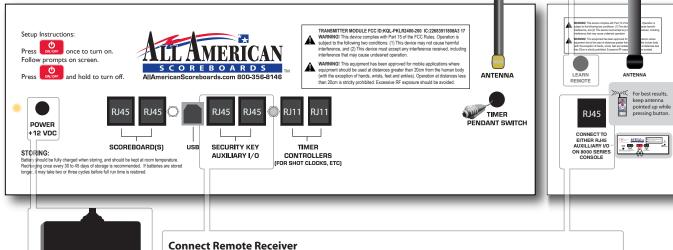
Connect Remote Receiver to either Auxiliary I/O connectors on the 8000 console. For best results, do not exceed 3' of CAT5 cable (supplied) between console and Receiver.
