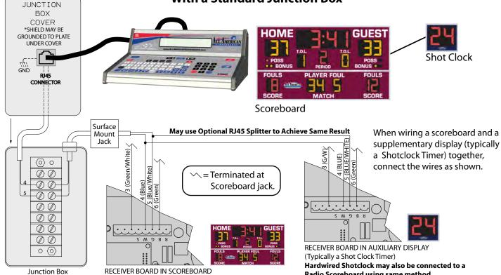
Single Scoreboard Wiring (Dual Box is Standard -See Dual Wiring Diagram) Radio Scoreboard using same method.
