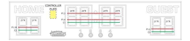
Power Supply Outputs (Full Brightness & Full Digits): P1.1≈3.42A P1.2≈2.60A P1.3≈2.81A P1.4≈2.81A
