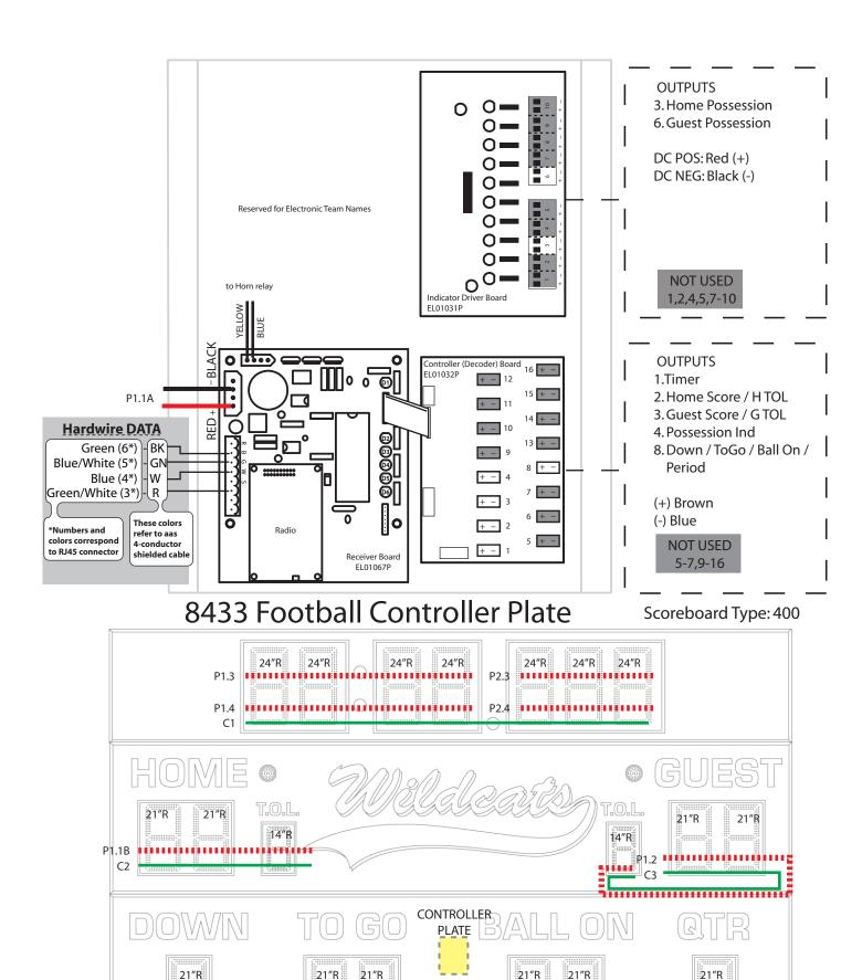
Power Supply Outputs (Full Brightness & Full Digits): P1.1≈4.23A P1.2≈2.81A P1.3≈2.81A P1.4≈3.57A P2.1≈3.90A P2.2≈3.90A P2.3≈2.11A P2.4≈2.11A
