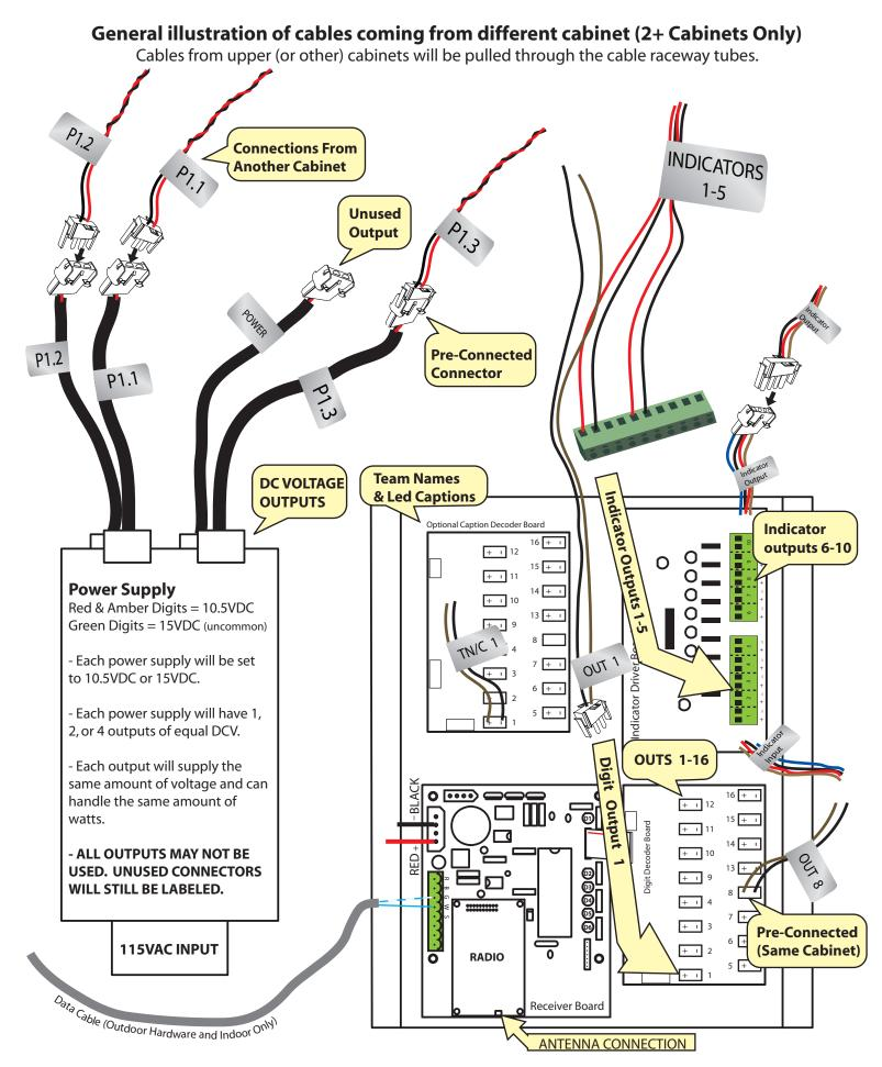
Sample connections - connections and hardware will vary depending on specific scoreboard. Cables from same cabinet will be connected. All Connections will be labeled. Large boards may have jumper cables - controller board may not need to be opened.
