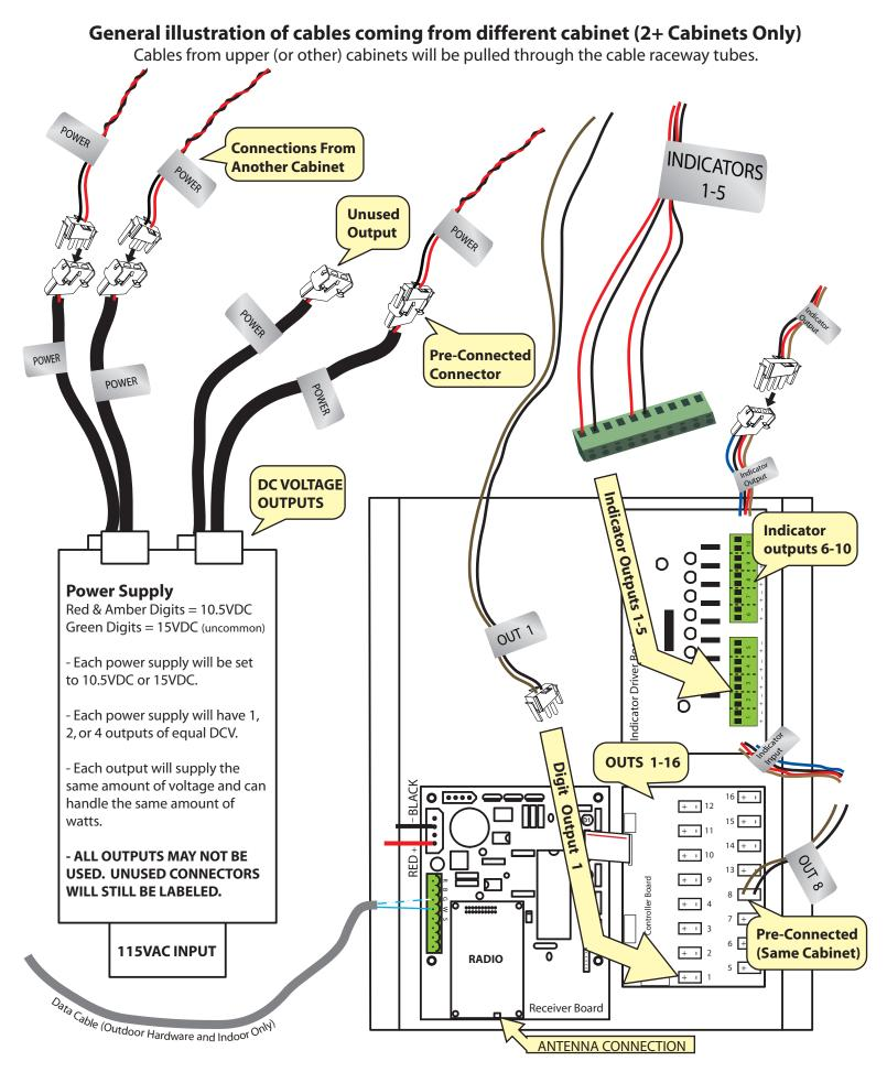
Sample connections - connections and hardware will vary depending on specific scoreboard.
