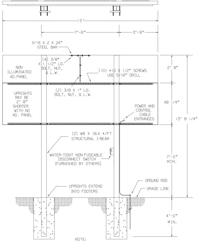
FOUNDATION SHOWN FOR ILLUSTRATION PURPOSES ONLY. ACTUAL FOUNDATION TO BE TO DESIGNED BY A REGISTERED ENGINEER TO MEET SITE SOIL CONDITIONS AND ALL APPLICABLE BUILING CODES
