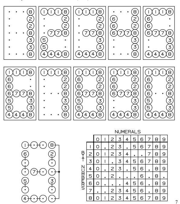
MICROPROCESSOR 4 X 7 (8 BIT) LED PATTERN
