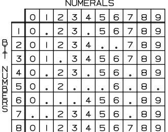
MICROPROCESSOR 4 X 7 (8 BIT) LAMP PATTERN
