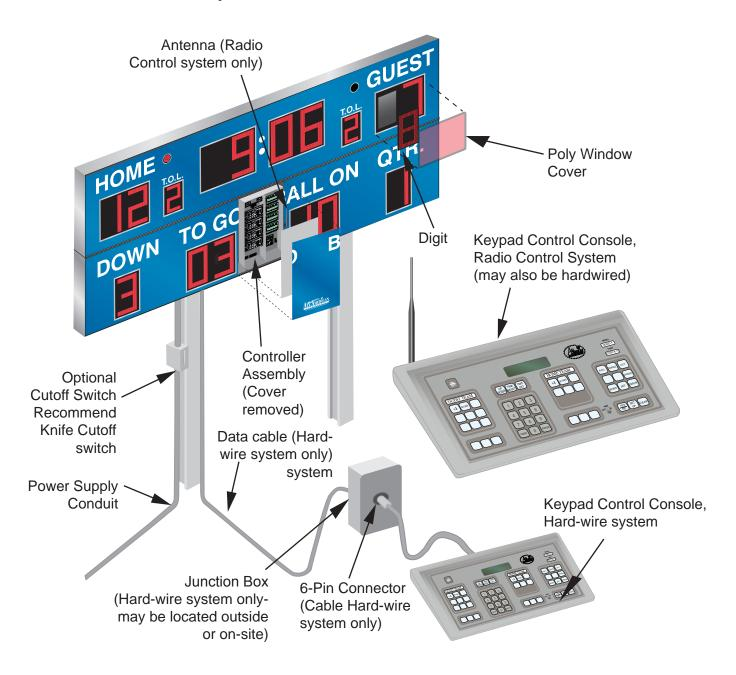
Figure 1: General Assembly of Scoreboard System (MP-7479 Shown)
