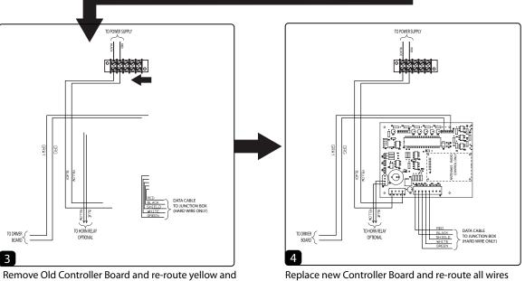
Remove Old Controller Board and re-route yellow and black wires on terminal block to connect to wires to Power Supply, yellow to red and black to black.
