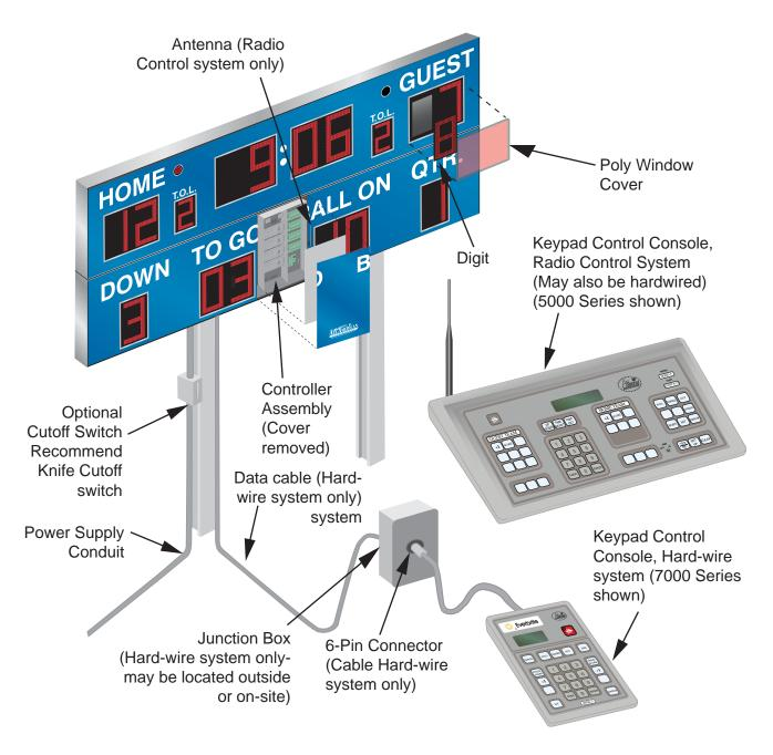
Figure 1: General Assembly of Scoreboard System (MP-7479 Shown)
