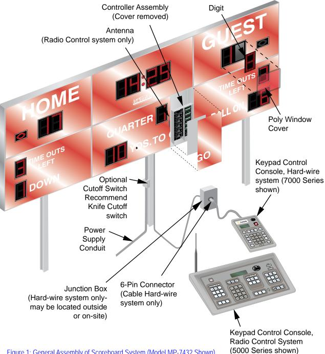
Figure 1: General Assembly of Scoreboard System (Model MP-7432 Shown)
