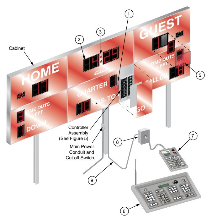
Figure 6: Assembly and Parts List
