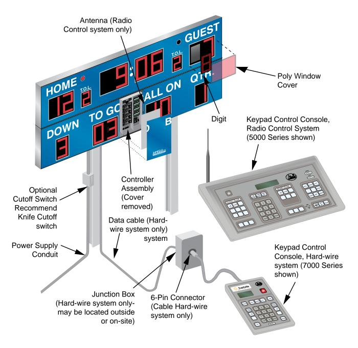
Figure 1: General Assembly of Scoreboard System (MP-7479 Shown)
