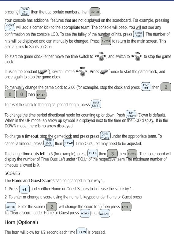
The horn will blow automatically at the end of each period for 2 seconds.
