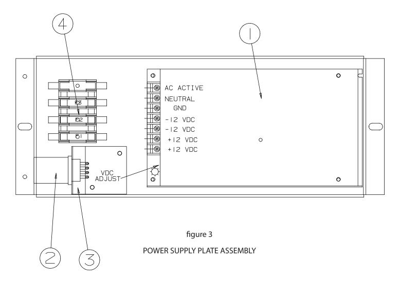
REPLACEMENT PARTS LIST Power Supply Plate Assembly
