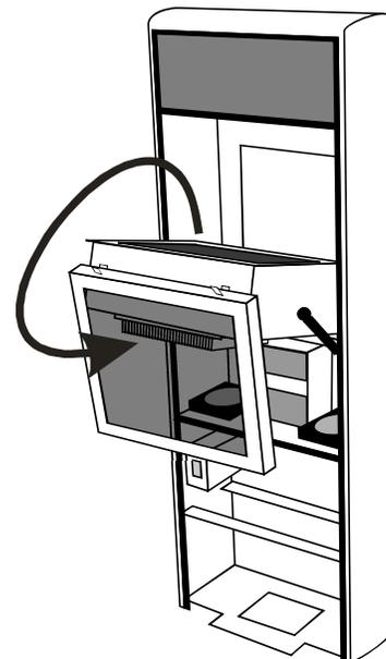
Step 6 Lift out the electronics insert and remove the old compact flash. Insert the new compact flash into the slot on the computer.
