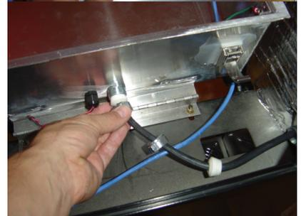
Step 23 Slide rubber washers, metal washers and nuts into place on the shell connector and tighten nut to seal connection.
