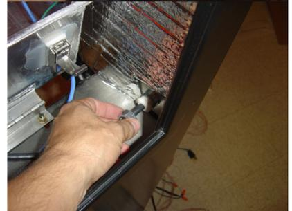
Step 24 Place ground wire from new heater/fan pan on closest mounting stud.
