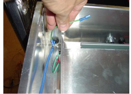
Step 26 Make sure heater/fan pan is pushed towards the bottom of the enclosure and secure ground wire using nut from step 8.
