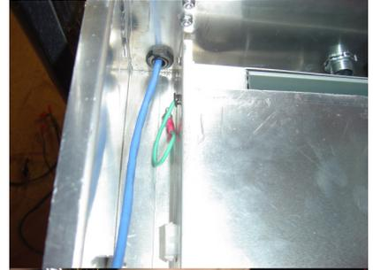
Step 25 Place ground wire removed in step 1 over same stud used in step 24.
