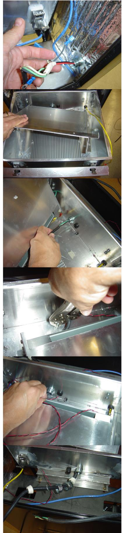
Step 20 Attach power cord to pull string and pull power cord from top to bottom so end is near switch box
