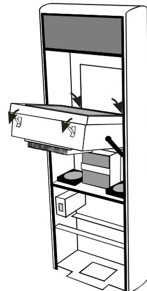
Step 5 Using caution not to twist the frame, lift off the face using the aluminum frame (may be tight) and leaving the ground strap in place, flip over the face so the holes in the frame can hang on the stainless steel face retainers.
