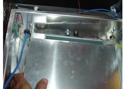
Step 22 Slide rubber washers, metal washers and nuts into place on the enclosure connector and tighten nut to seal connection.
