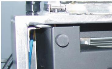
10. Slide the electronics insert back into the internal enclosure between the bottom of the box and the two retaining brackets which hold it in place (see image right).
