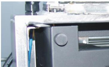
10. Slide the electronics insert back into the internal enclosure between the bottom of the box and the two retaining brackets which hold it in place (see image right).
