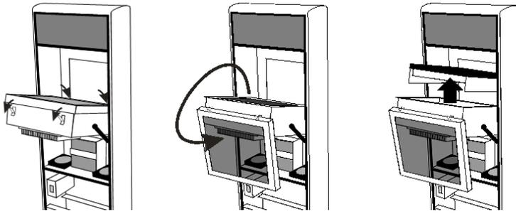
4. Release the four face retainer latches (two are in front & two are in back).
